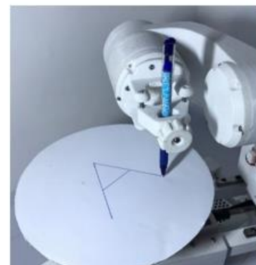
Figure 14 - Robot manipulator plotted test drawing (with attached pen plotting tool)
