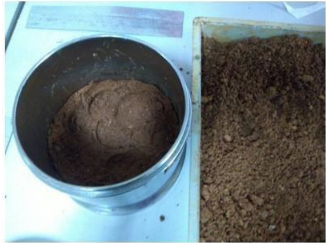
Image 09 & 10- Sample preparation of CBR Test
