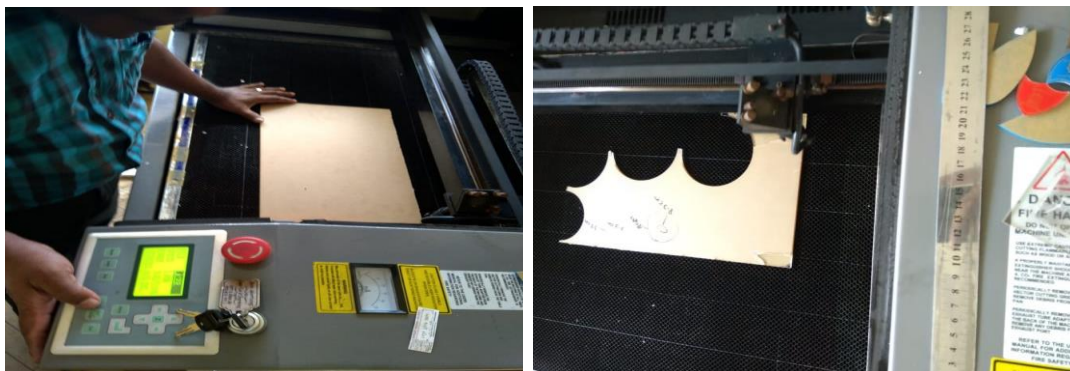
Figure 4: laser cutting of Acrylic Sheet Clear Plexi plastic board
