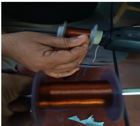
Figure 1: Coil Winding using drilling machine Figure 2: Coil winding on a handmade cardboard
