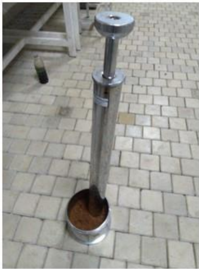
Image 09 & 10- Sample preparation of CBR Test
